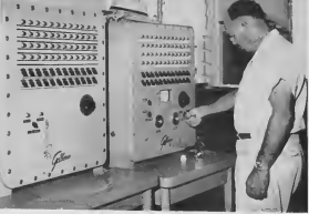
CRUDE FIELD operator Ronald Clauzel flips the calibration switch on the Gilbarco main receiver to check crude level in one of 27 crude tanks so far incorporated in the automatic gauging system. OPERATOR DEN Crude Field Ronald Clauzel in flip a calibration switch arbi e Gilbarco sa receptor mayor pa check nivel di e crudo den e di 27 tankinan cu ya ta inclui den e sistema automatico di gauging.
